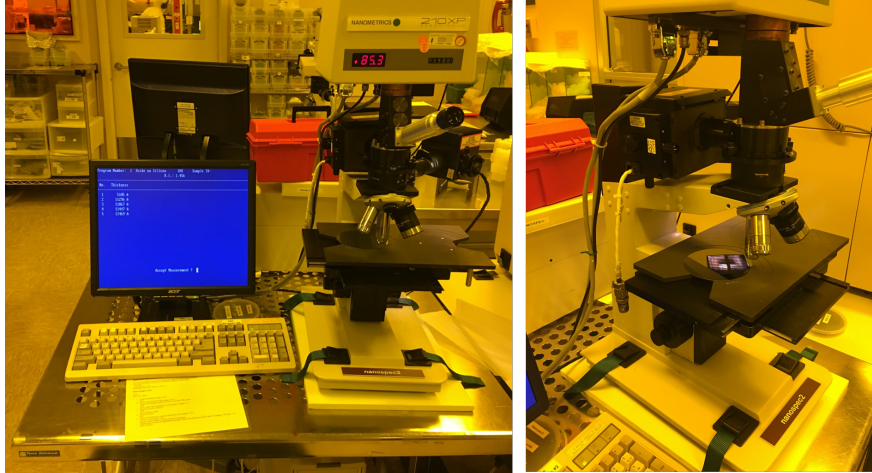
Figure 5: (Left) The NanoSpec 210XP system used to confirm the SiN thicknesses resulting from the Thermo-coNitride deposition. (Right) A closer view of the facility demonstrating the silicon calibration wafer to be used before any measurement.
