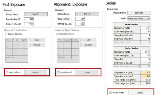
Figure 14: Unloading options in Standard Mode and Series Mode
