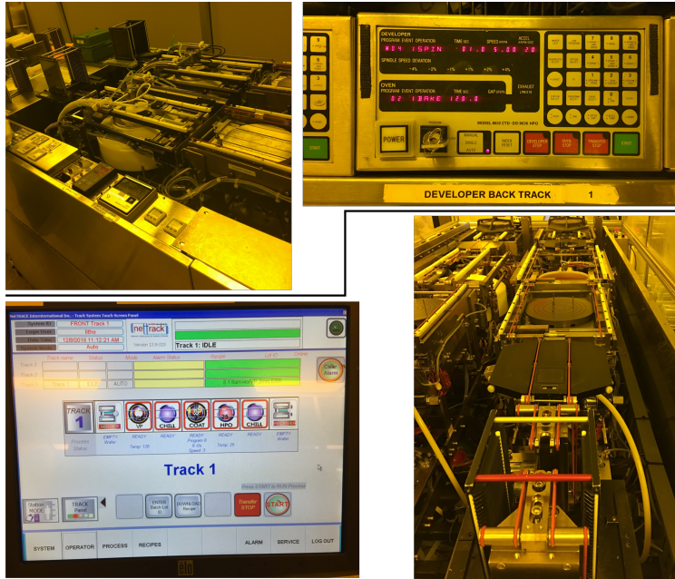
Figure 9: (Top row) The SVG Developer tool, and (bottom row) The SVG Coat tool.
