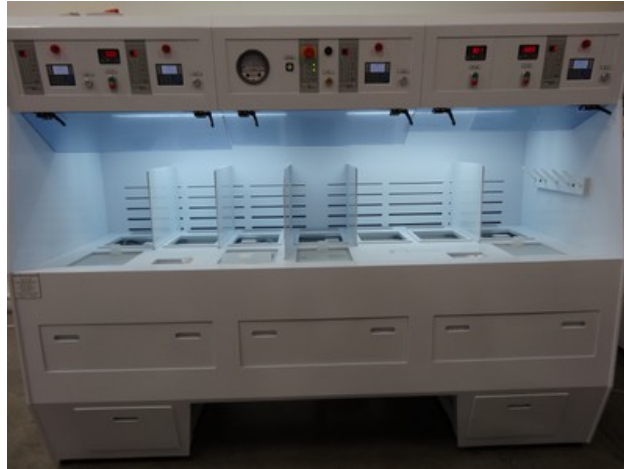
Figure 3: The wetbench clean facility that ensured the removal of surface imperfections and organics. This was performed shortly before the silicon nitride deposition. Adapted from the SNF wiki.
