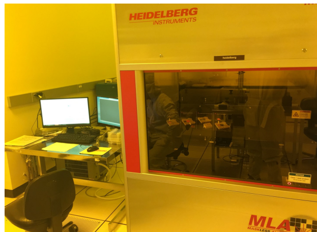
Figure 10: The Heidelberg MLA150 maskless lithography system was used to directly expose the grating features over the 1\mu\text{m} 3612 photoresist on top of the silicon nitride wafer.
