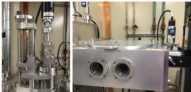
Figure 21: (Left) The chuck alignment controls for aligning the AJA evaporator chuck, as well as (Right) the load lock where the chuck containing test wafers is placed.
