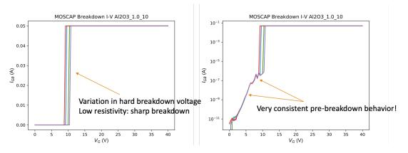
c. For MOS structures, you may see less sharp breakdown behavior depending on the resistivity of the substrate and the exact doping profile
