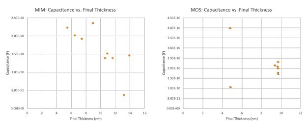
Capacitance is extracted from low-frequency (1kHz) C-V curve @ 1V
