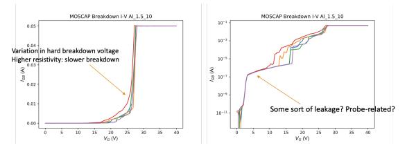
d. In either case, you can expect to see variation in the breakdown threshold voltage due to intrinsic variations in the breakdown behavior device-to-device
