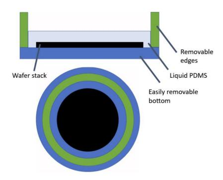
Fig. 1 – Front (top) and top-down (bottom) views of a schematic of the mold. The blue material is a flat ceramic tile, the green material is the polymer clay, and the black material is the wafer sample.
