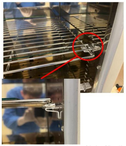
Fig. 2 – Levelling an oven shelf using little squares of aluminum foil to achieve a perfectly flat surface for curing the molded PDMS.
