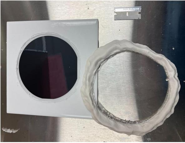
Fig. 3 – Using the blade, cut around the perimeter of the PDMS, then gently pull the clay up and away from the ceramic tile.
