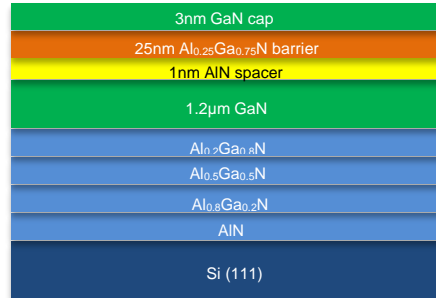
Fig. 5 GaN-on-Si HEMT structure
