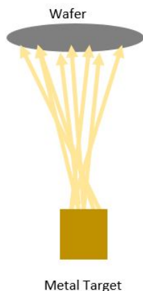
Figure 4: Schematics of a sputtering metal deposition system
