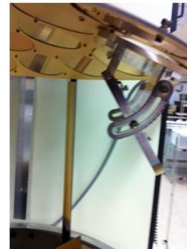
Figure 3: Angled mount configuration that we used in Innotec for our depositions
