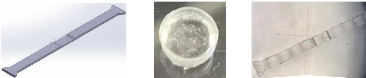
Figure 9: (a) Microchannel mold (b) PDMS with embedded microchannel structure (c) Microchannel Structure inside PDMS
