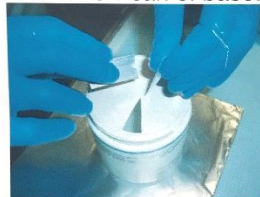
Make pouring and venting cuts
