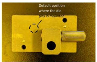
Currently the tool has an X-shifter that can shift the die to your right by 7.5 mm, and 7.5 mm downwards.
