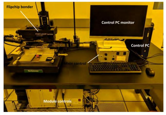
Flipchip bonder: this is the functional component of the tool
