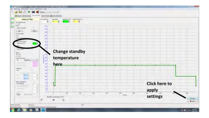
ii. For CCH module, go to tab "CCH Module", change the standby temperature under section "Heating Plate Standby", and click "Apply" at the bottom right corner to apply the settings.
