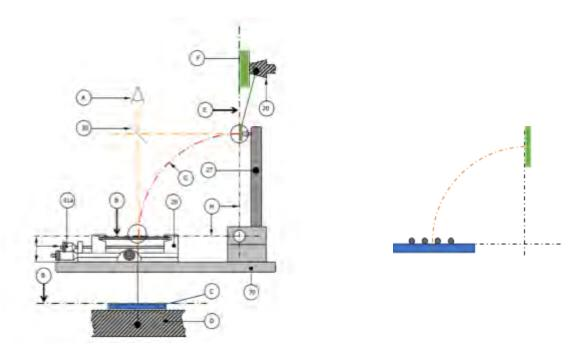
The key capability of the flipchip bonder is to align (in x, y, and z) between the die and the substrate. The main components of the tool are a table that holds the substrate and can be adjusted in x, y and z directions, and a movable arm that holds the die.
