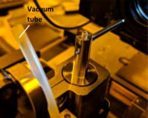
→ After the die pick is inserted, do not yet tighten the screw. First connect the vacuum tube to the back of the die pick.
