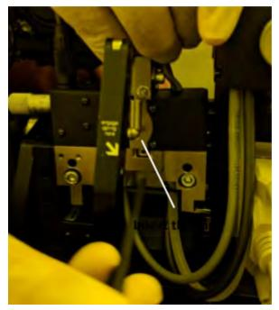
9. Take out the ultrasound die pick from its storage tube, and insert it into the hole on the transducer. If the die pick cannot be
