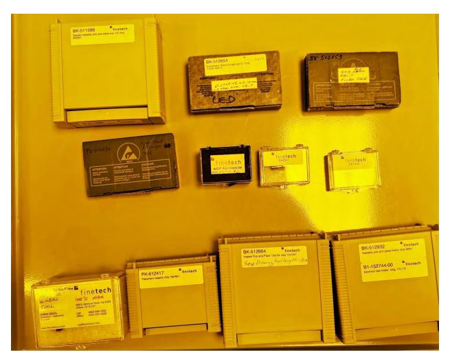
The pictures show the various **die pickups** and **X-shifters** that are avaialble for the tool. The positions of the components in the first picture match that of their containers in the second picture.
