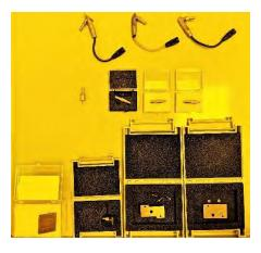
**CAUTION:** do **NOT** change the die pick if the tool is turned on. You may burn yourself as the die pick is heated to standby temperature when the tool is turned on. Changing the die pick should ALWAYS be done when the tool is turned off.
