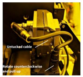
2. To disconnect the mounted die pick, first untuck the tucked cable from under the base. Then release the cable connector, by rotating the grooved ring on the cable connector counterclockwise to the unlocked position and pulling up the connector.
