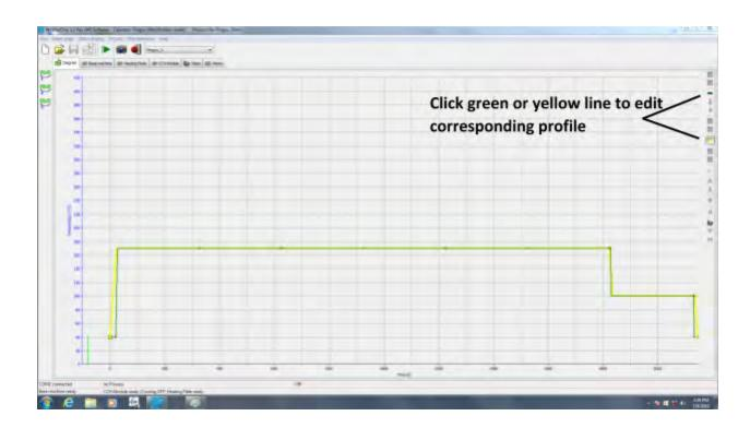
The temperature profile consists of several segments, each defined by three parameters: ramp rate (K/s), plateau temperature (°C) and duration (s). The parameters can be edited by
