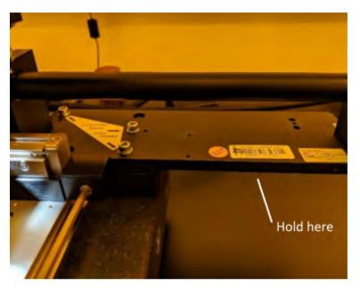
10. To install the other force arm, place it in position, with the three screw holes on the force arm matching the holes on the tool, and the two holes on the force arm matching the screws on the tool.
