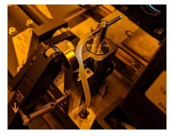
Attach the cable holder for the ultrasound module to the tool. Install the holder to the screw hole indicated on the right.
