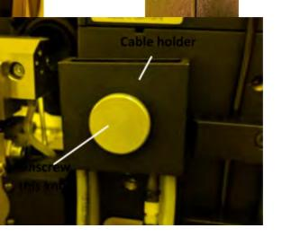
4. → Unscrew the cable holder from the tool, by rotating the knob counterclockwise. Once the cable holder comes off, set it aside on the table.
