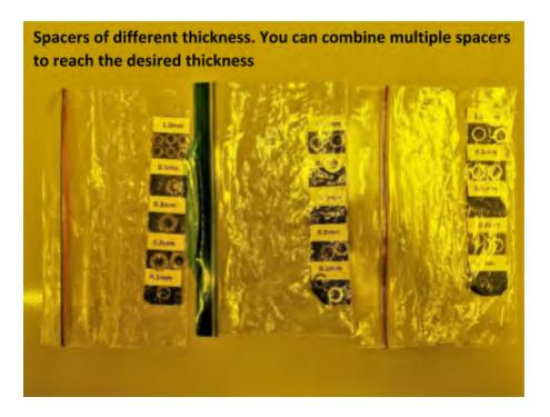
The spacers go to the back of the die pick. To add a spacer, slide it down the rod that mounts the die pick to the base.
