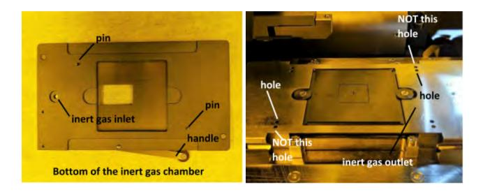
Once installed, you can use the handle to open and close the lid. Open the lid when loading the substrate, and close the lid during alignment, contact, and bonding. For best inert environment, with the lid closed, let the nitrogen flow for several minutes before the bonding process.
