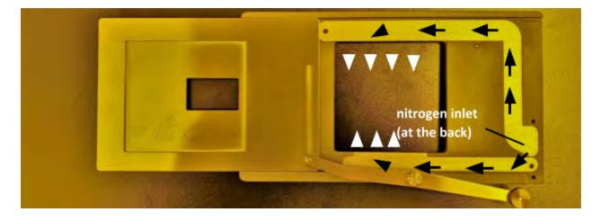
To install the inert gas chamber, with the handle facing toward you, align the pins at the bottom of the chamber to the holes on the heating plate. If properly installed, the inert gas chamber will sit onto the heating plate firmly.
