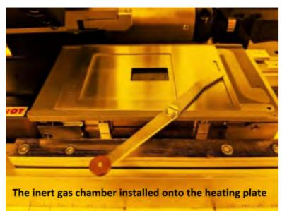
Nitrogen is flown into the chamber through the tracts shown below. By constantly flowing nitrogen and closing the lid, the remaining air inside the chamber is pushed out from the window on the lid, and an inert environment is established. The picture below shows how the inert gas is routed and flown into the chamber.
