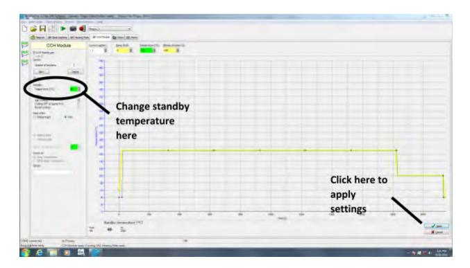
Set up the temperature profile. The "Diagram" tab shows the temperature profile (yellow trace: chip heating contact module; green trace: heating plate) for the bonding process. To edit the profile, click on the corresponding colored icon on the right.
