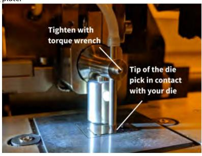
**CAUTION**: if you have dies of different thickness, make sure to perform the calibration, using the die that you plan to bond, **every time** before you do the bonding process.
