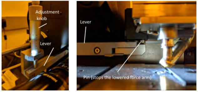
The default position on the knob is marked by a black line, which is 1.61. Default position means that there is no gap between the die and the substrate. Rotating the knob counterclockwise decreases the gap distance, and clockwise increases the distance.
