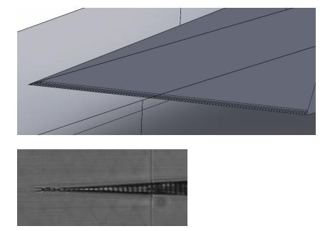
Rough edge: 5 µm wide, 1 µm tall. Blade made with 63x. Doesn't come out at 25x
