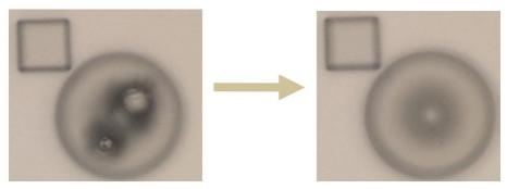
Figure 2. Preheat is a useful tip to reduce bubble formation in writing.
