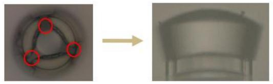
Figure 1. The less tension drying methods improve the mechanical stability of the overhanging structures.
