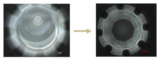
Figure 6. An off-center issue could be avoided by combine two GWL files with a different writing direction.
