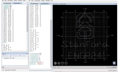
Figure 7. An example of using a simple GWL code to draw a Stanford Logo.
