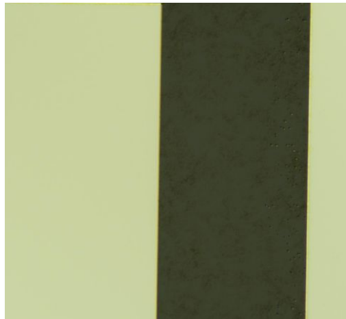
Figure 1. Microscope picture of post-metal etch residue on sapphire between two Nb areas
