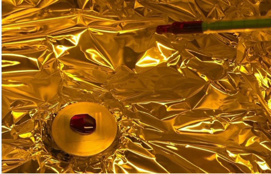
Figure 5: Deposition of SPR220-7 onto ITO coverslip with a syringe
