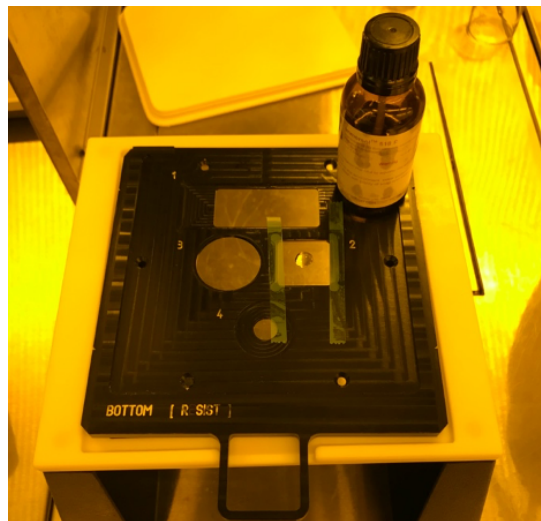
Figure 3: Deposition of immersion oil on the BOTTOM side of the substrate
