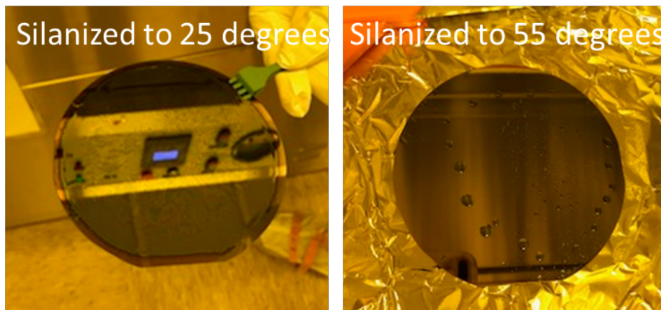
Figure. Hydrogel spin coating on thermal oxide on silicon wafers.
