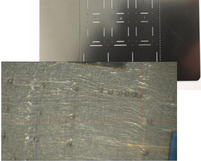
Left - stencil purchased for project Right - close up optical image of solder paste stuck in apertures of our stencil
