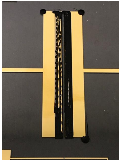
Figure 6 Alignment of pre-existing features on a glass substrate. Circles on the corners were used to align the probe with the alignment marks
