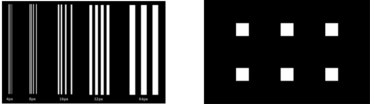
Figure 17: Images used to assess pattern quality in microfluidic channels. Column widths ranged from 4 pixels ( \sim 1.1\mu\text{m} ) to 64 pixels ( \sim 17.6\mu\text{m} ). Square boxes were 140 pixels across ( \sim 38.5\mu\text{m} ).
