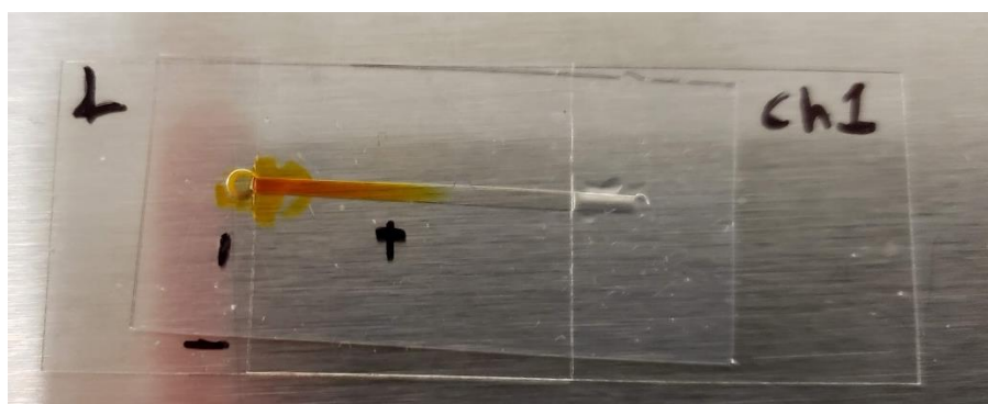
Figure 24: Channel formed with glass coverslip filled halfway with PLPP (right) and a mixture of PLPP and yellow dye (left)
