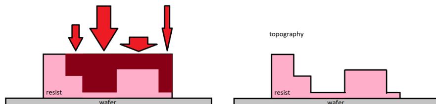
Fig 2: Grayscale lithography on a positive photoresist
