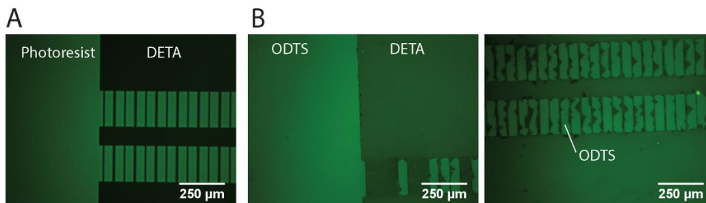
Figure 10: Fluorescence test of patterned organosilane (A) The fluorescence background of photoresist and DETA. (B) FITC coating on the wafer after lifting off photoresist. The high intensity of fluorescence in ODTS area showed that the photoresist was not totally removed.
