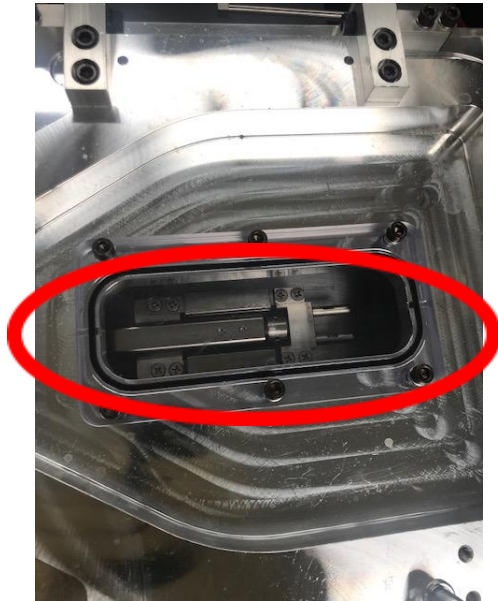
Figure 2: View of transfer fork through loadlock window
