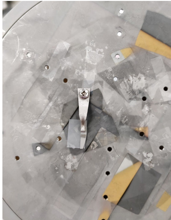
Figure 2. Shows mounting procedure for high temperature depositions
