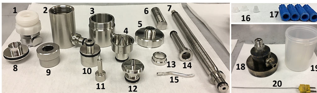
Figure 13: Optomec parts that require thorough cleaning. Critical parts: 4, 6, 7, 8, 10, 11, 12. Critical parts that cannot be cleaned with Branson: 18.
