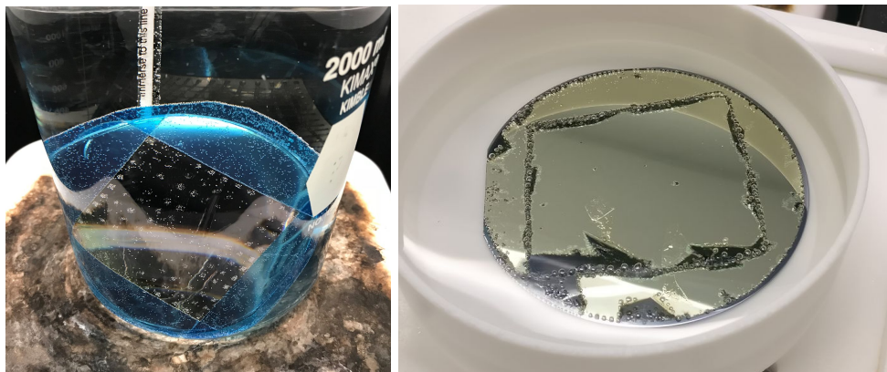
Figure 2. Wet etch, Ge-H 2 O (left) and Al-HF (right); stiction and bubble were the issues of wet etch.
