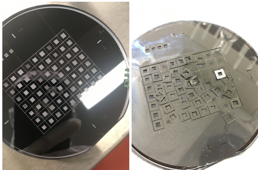
Figure 4: A wafer before (Left) and after (Right) device lift off.
