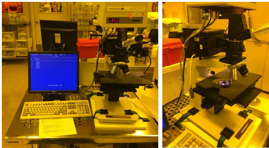
Figure 8: (Left) The NanoSpec 210XP system used to confirm the nitride thicknesses resulting from the ThermcoNitride deposition. (Right) A closer view of the facility demonstrating the silicon calibration wafer to be used before any measurement.
