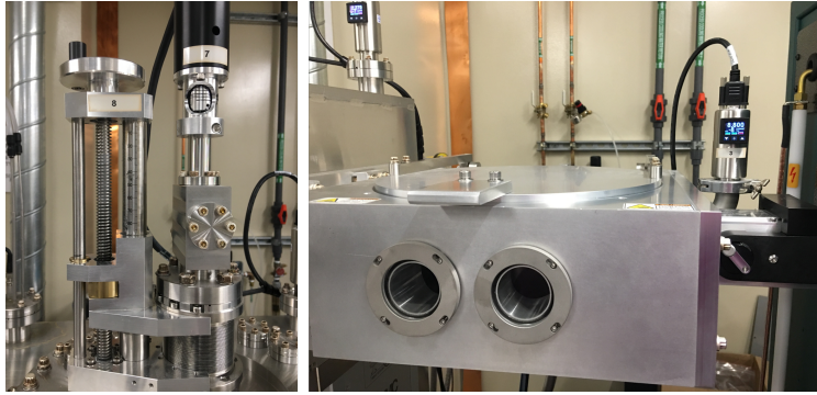
Figure 18: (Left) The chuck alignment controls for aligning the AJA evaporator chuck, as well as (Right) the load lock where the chuck containing test wafers is placed.
