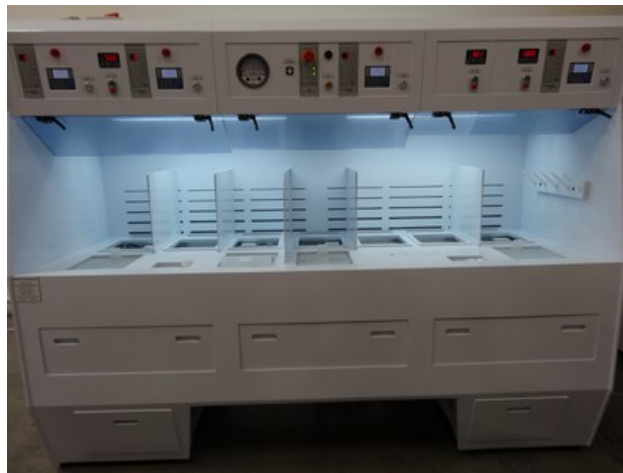
Figure 5: The wetbench clean facility that ensured the removal of surface imperfections and organics. This was performed shortly before the silicon nitride deposition. Adapted from the SNF wiki.
