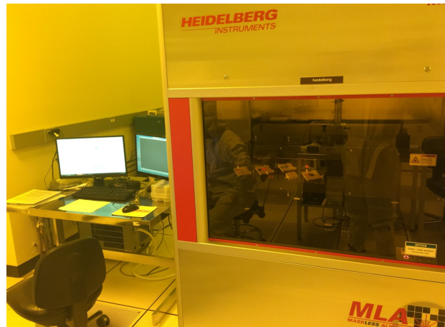
Figure 13: The Heidelberg MLA150 maskless lithography system was used to directly expose the grating features over the 1\mu\text{m} 3612 photoresist on top of the silicon nitride wafer.
