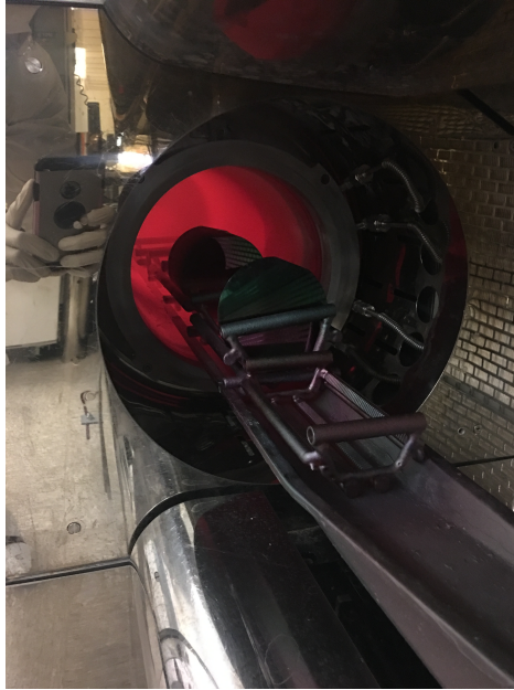
Figure 7: The ThermcoNitride tube "boating in", or being slowly inserted in the furnace to begin deposition and avoid thermal shocks.
