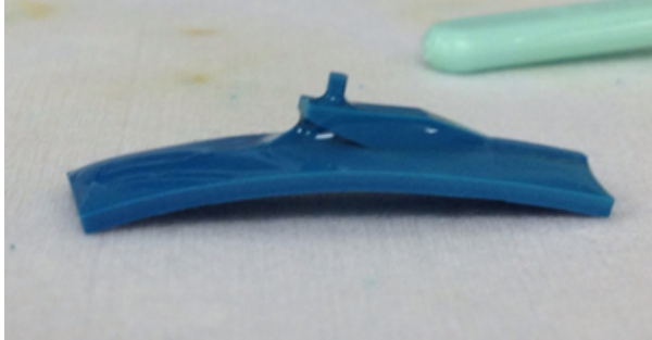
Warping of a mold improperly post-processed.
