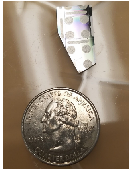
Figure 12.) InAlN/GaN Hall effect test structure
