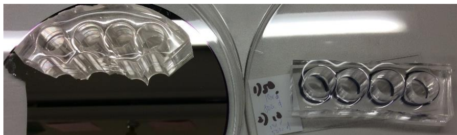
Fig. 2: Functionalization setup for Pt film on Si wafer (left) and glass slide (right)
