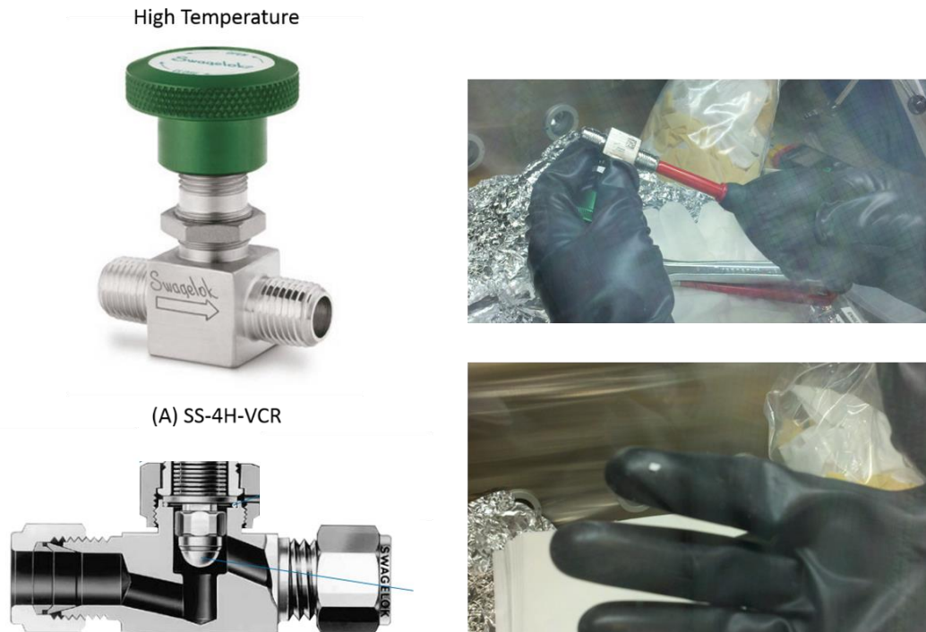
Figure 6: High temperature manual valve and cross section. A pellet formed by clogging in the bellows region is also shown.
