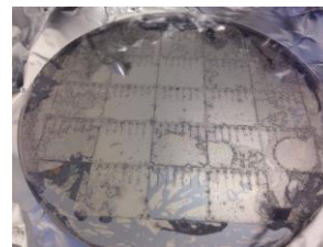
Fig. 7: Wafer stack after curing process, using with liquid glass as adhesive
