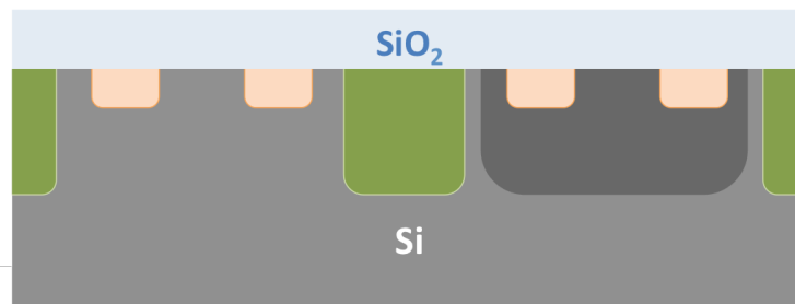
Figure 6. A flash anneal is performed to drive in the implants.
