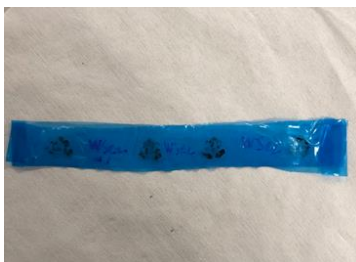
Fig 10. A blue exfoliation tape containing WSe 2 crystals, prepared from a bulk WSe 2 crystal
