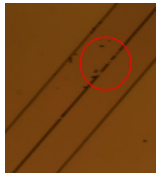
Figure 38: Broken waveguide from Attempt #1
