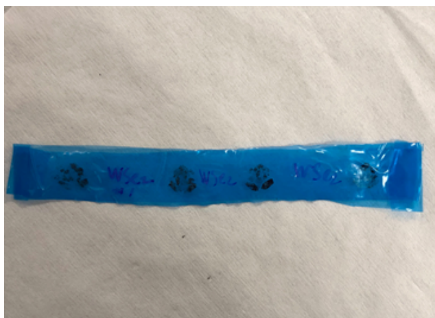
Fig 1. A blue exfoliation tape containing WSe 2 crystals, prepared from a bulk WSe 2 crystal
