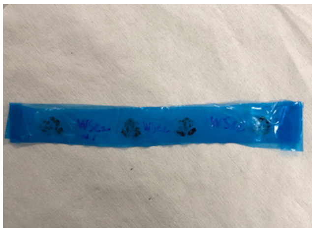
Fig 12. A blue exfoliation tape containing \text{WSe}_2 crystals, prepared from a bulk \text{WSe}_2 crystal
