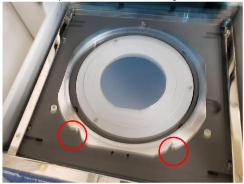
6. Pull out the tape and completely cover the wafer and the metal ring. Make sure the tape is affixed to the side rails.
