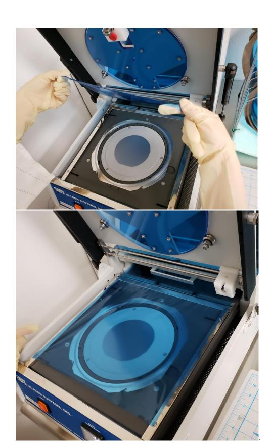
7. Pull out the roller tool and roll to smoothen out the tape and ensure proper adhesion to the backside of the wafer. If there are any bubbles present, remove them using the plastic smoothening hand tool.
