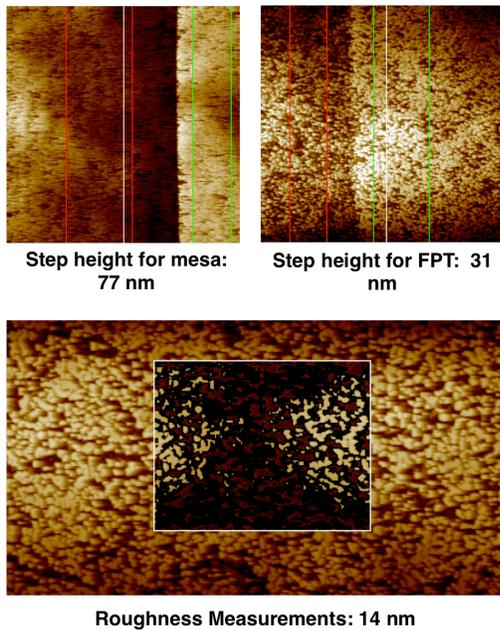
Figure 9: AFM measurements of mesa step height, FPT step height, and AlGaIn wafer roughness
