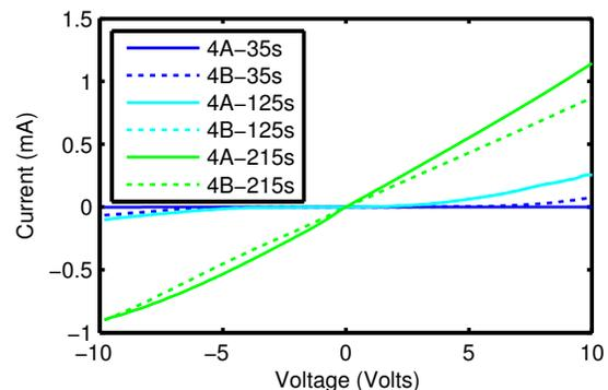
Figure 5: Graph of how increased anneal time effect current-voltage response of multiple devices on a die
