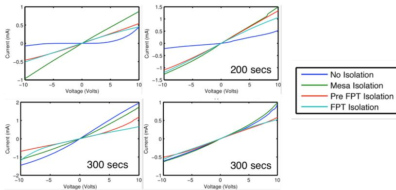
Figure 7: Comparing isolation techniques and device performance before and after FPT
