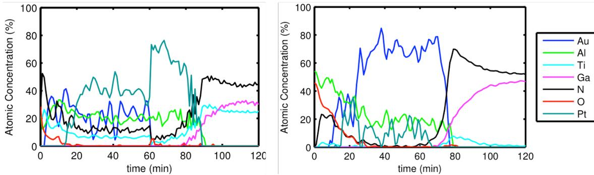
Figure 6: Graphs of atomic concentration with sputter time as surface is slowly removed via argon sputtering for single RTA (35 seconds) sample (left) and a sample with a total RTA time of 215 seconds (right).
