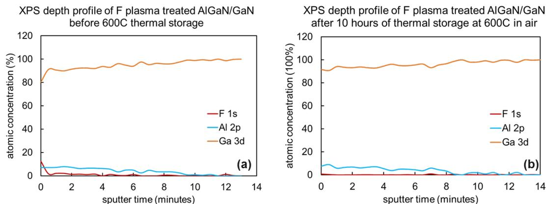
Figure 10: XPS depth profiles incorporated fluorine of FPT AlGaIn/GaN samples before and after 10 hours of thermal storage at 600C in air.
