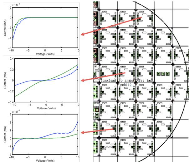
Figure 4: Schematic illustration and graph depicting nonuniformity of current voltage response across the wafer
