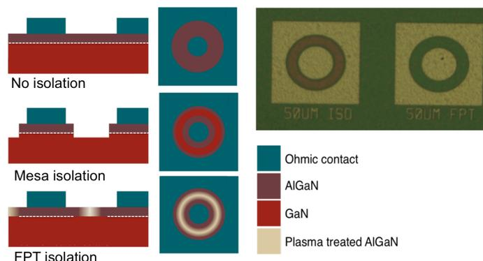
Figure 1: Schematic illustration cross section and optical image of top view of circular test structures with no isolation, mesa etch isolation, and FPT isolation.
