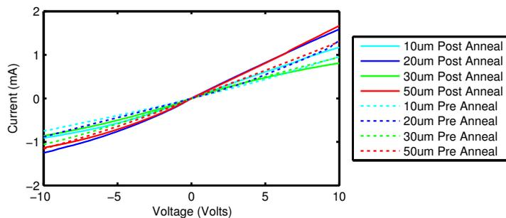
Figure 8: Comparing FPT performance before and after 10 minute, 600C anneal in nitrogen
