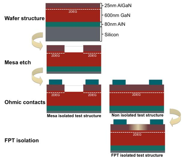
Figure 2: Schematic of isolation test structure fabrication process
