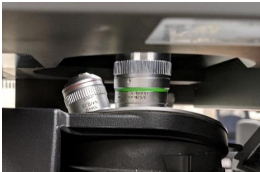
Figure 19: Correction collar: Default value for glass coverslip is indicated with a black mark
