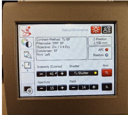
Figure 20: Image of the Leica microscope control panel with transmitted light (TL) shutter open and brightfield light intensity set to 41%.
