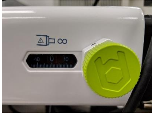
Figure 24: Tube Lens Adjustment Knob (located on the side of the PRIMO optical case)
