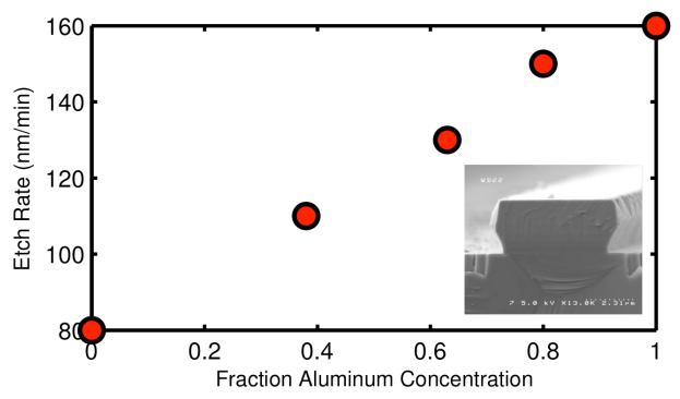
Figure 9 Lateral etch rates (parallel to 0001 crystal plane) in 200°C 3:1 sulfuric/phosphoric acid for the AlGaN/GaN HEMT layers varied with Al%. Inset is an SEM image of sample used for measurements.
