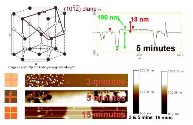
Figure 3 (Top Left) GaN Wurtzite lattice, with 1012 plane drawn in dark red. (Top Right) AFM profile of ALN sample etched in phosphoric acid at 150 °C for 5 minutes with both C plane etching and large defects profiles. (Bottom) Optical and AFM images of AIN features etched for 3, 5, and 15 minutes from top-bottom. These show a defect-drive etch mechanism.
