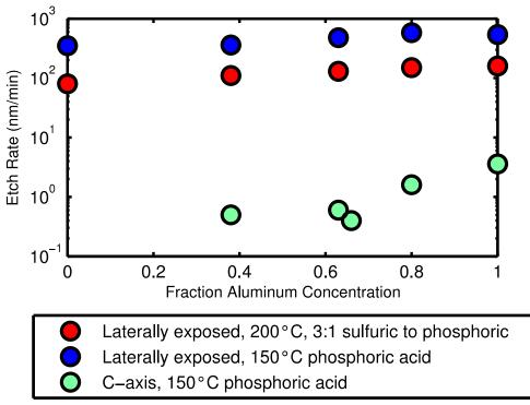
Figure 11 Summary of the vertical and lateral etch rates of GaN, AIGaN, and AIN with respect to aluminum concentration for phosphoric acid and sulfuric/phosphoric acid.
