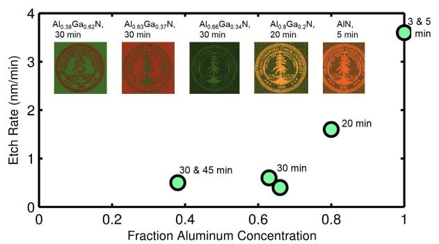
Figure 5 C-plane (vertical) etch rates of AlGaN sampled with varied Al concentration. Insets show optical images of AlGaN sampled etched with Stanford logo pattern. The data points are annotated with the etch time for each sample measurement – the window of time varies.
