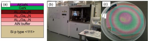
Figure 12 (a) Cross section of HEMT wafer films when grown on Si. (b) Image of the AAxitron metalorganic chemical vapor deposition system (MOCVD) (c) Image of the grown HEMT wafer.
