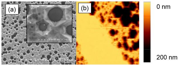
Figure 4 SEM of AIN sample etched for 5 minutes in 150 °C in phosphoric acid with inset of higher magnification, revaling hexagonal etch pits. (b) AFM image if the same AIN sample.
