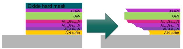
Figure 6 Schematic illustration of measurement method used to characterize lateral etch. The AlGaN/GaN HEMT layer was plasma etched in Ox III-V and then wet etched in a wet phosphoric etchant, revealing the anisotropic etch rate of the III-nitride films. The AIN buffer was hypothesized to etch faster in plane than the (AI)GaN layers.
