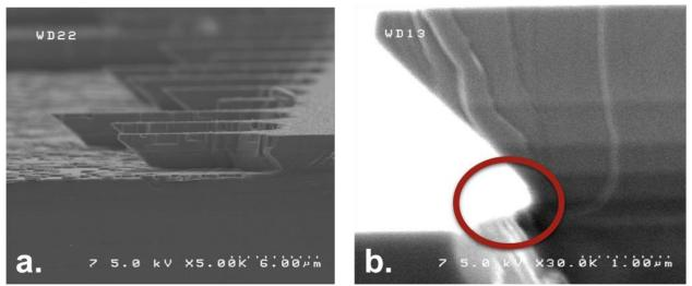
Figure 10 (a) SEM image of a pre-released cantilever array etched in 150 °C phosphoric acid for 5 minutes. (b) SEM image of a HEMT structure with undercutting also etched in 150°C phosphoric acid for 45 minutes, revealing an AIN crystal plane with different dominant etch plane(~21°).
