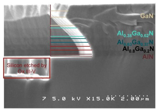
Figure 7 Cross section of the AIGaN/GaN HEMT structure used for lateral etching characterization. This cross section is from the sample that was etch in 3:1 sulfuric/phosphoric acid. The dips into the silicon substrate on the bottom left are artifacts from the plasma etch step, and can be used as a reference line to measure lateral etch rates of each film.
