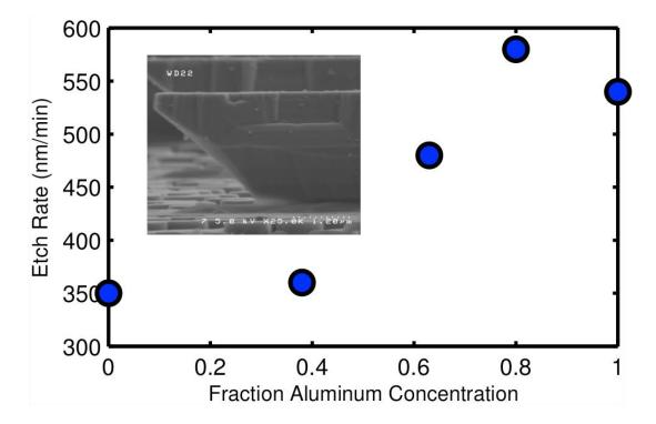
Figure 8 Lateral etch rates (parallel to 0001 crystal plane) in 150°C phosphoric acid for the AlGaN/GaN HEMT layers varied with Al%. Inset is an SEM image of sample used for measurements.
