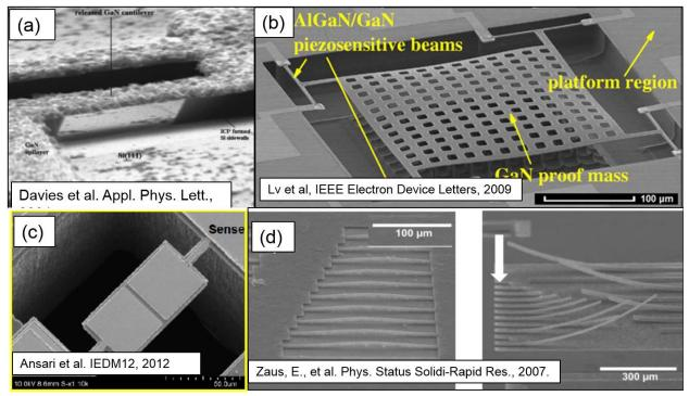
Figure 1 Previous work in the release of GaN and AlGaN/GaN films. (a) MBE GaN/AIN on Si released by Si dry etch and KOH undercut. (b) MOCVD AlGaN/GaN/AIN on Si released by SF<sub>6</sub> + O<sub>2</sub> plasma undercut. (c) MOCVD GaN/AIN on Si released by backside Si ICP etch.(d) MBE GaN/AIN on sapphire released by H<sub>3</sub>PO<sub>4</sub> wet etch
