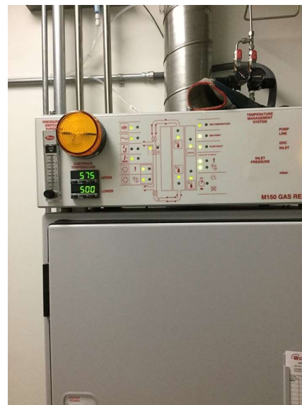
Figure 7: Scrubber with the temperature gauge
