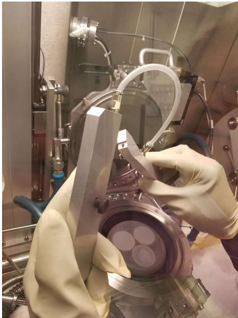
Figure 25: Gas flow dispenser
