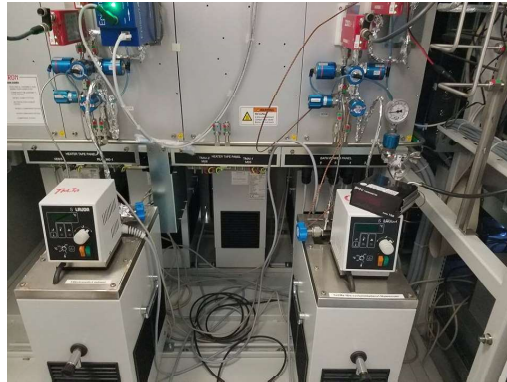
Figure 13: Bubbler thermostat to set and measure temperature
