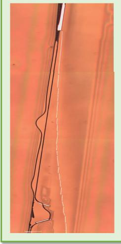
Shearing of long thin wires due to **nonuniform pressure** applied by clamp
