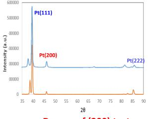
Degree of (200) texture seems to increase with O<sub>2</sub> fraction & pressure W9: 7.8 mTorr, 2.5% O<sub>2</sub>, 30 °C
