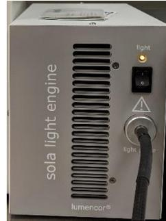
**Step 2:** Turn on Sola Light Engine: First turn on the power switch (located in the back) then turn on the light switch
