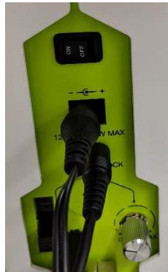
**Step 4:** Turn on the PRIMO laser controller: First turn on the power switch (located in the back) then turn the key clockwise to on position
