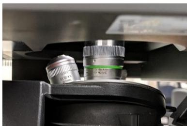
Figure 5: Correction collar. Default value for glass coverslip is indicated with a black mark
