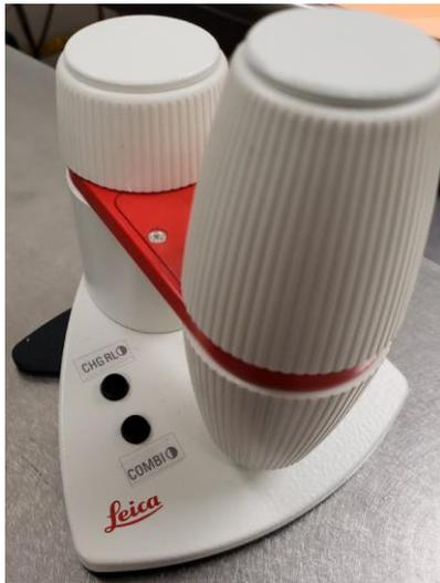
Step 2: Use the CHG RL button on Leica controller to adjust the Infinity Port setting (incoming light source) from Rear (PRIMO module) to Side (Sola Light Engine). The output port should remain set to Left (camera) or Eyepieces (if viewing manually).
