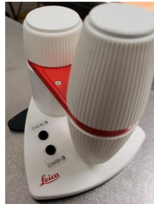
Step 4: If Infinity Port is set to something other than Rear (i.e. Side), toggle using the CHG RL button on the Leica controller
