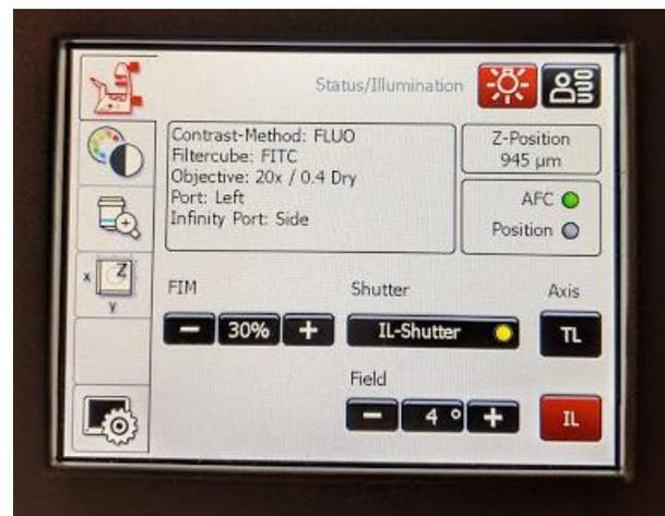
Step 3: Final microscope settings for fluorescent imaging. **As a courtesy to other users, please return the Infinity Port setting to Rear once imaging is completed.**
