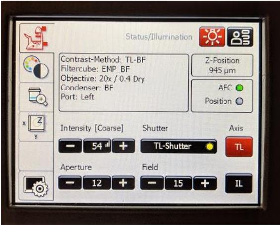
Step 1: Default microscope settings for patterning with the PRIMO laser diode (using the dedicated PRIMO EMP\_BF filtercube)
