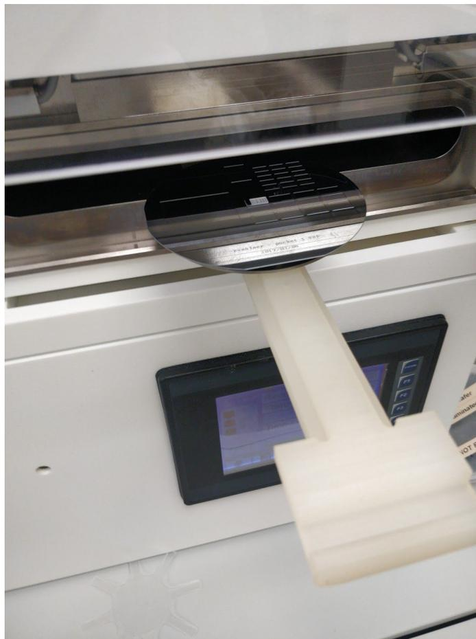
*Figure 16. Image of our carrier wafer with a chip placed in one of the inserts. This chip is 5mm x 10 mm. The carrier wafer is a silicon wafer processed to have 1800 micron deep inserts of several dimensions.*
