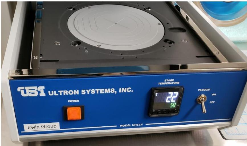
3. For best adhesion, **wait** until the stage temperature reaches the set point (50°).
