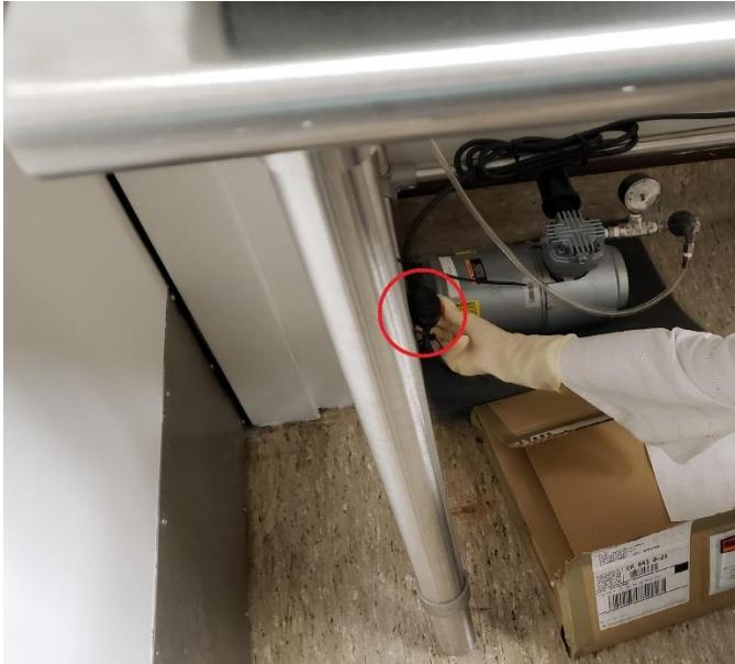
2. Turn on the machine using the orange power switch. Then, turn on the vacuum using the silver switch labelled “vacuum.”
