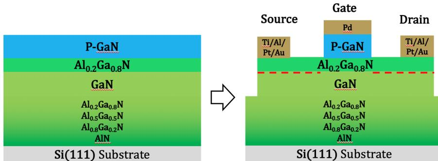
Figure 4: P-GaN/AlGaIn/GaN HEMT with Suppressed 2DEG for Zero Bias
