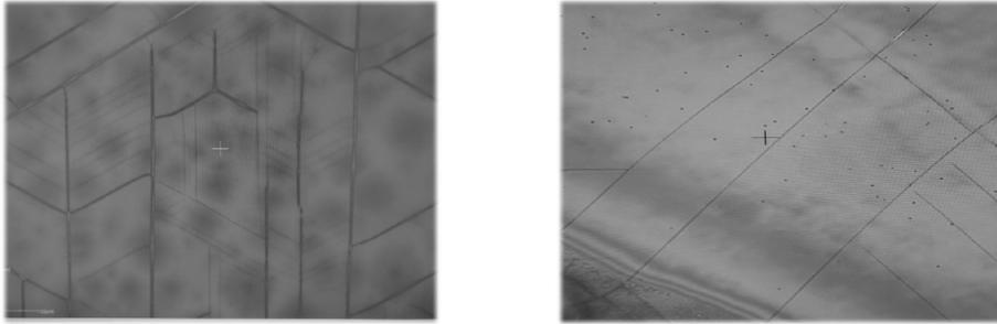
Figure 5: Cracks seen on the surface of gallium nitride samples after the MOCVD growth using Stanford aix-ccs
