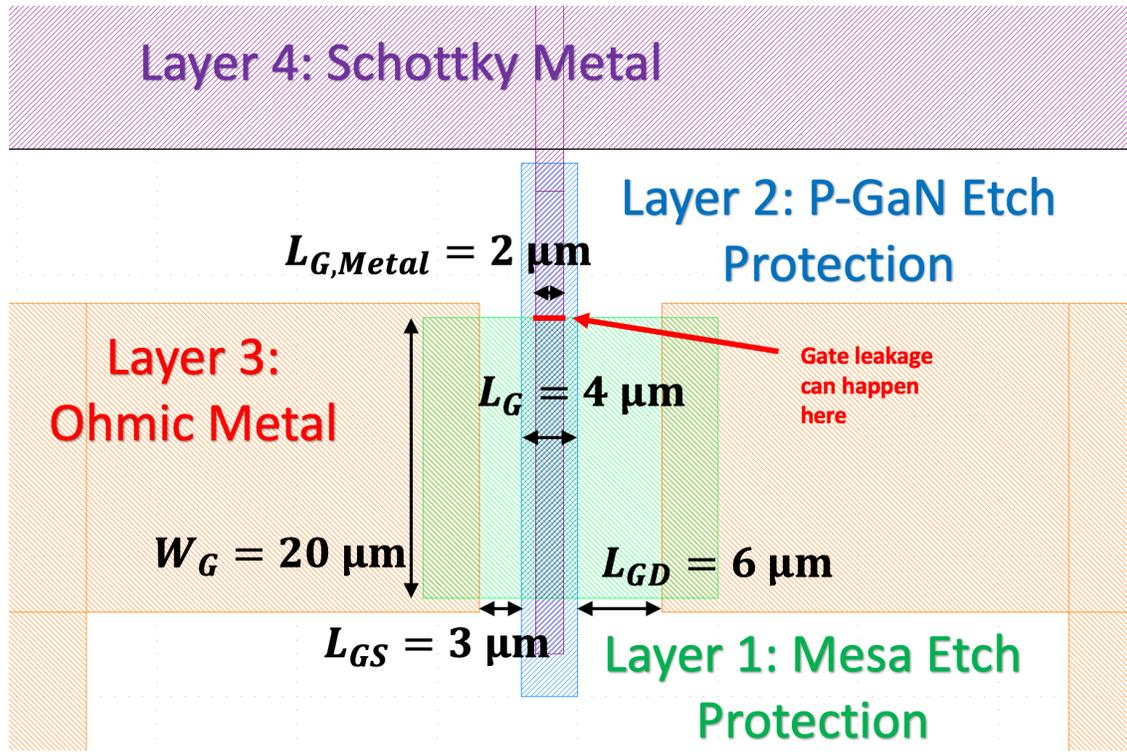
Figure 7: Example mask design for the P-GaN E-mode HEMT. It consists of 4 layers in total: (1) Mesa etch protection (2) P-GaN etch protection (3) Ohmic metal for S and D (4) Schottky metal for G. We will discuss it later, but the red line is where the gate leakage is likely to happen.
