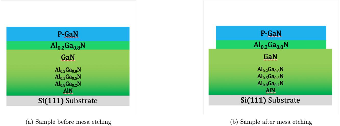
Figure 9: Mesa etching to leave AlGaIn/GaN heterostructure only for active area
