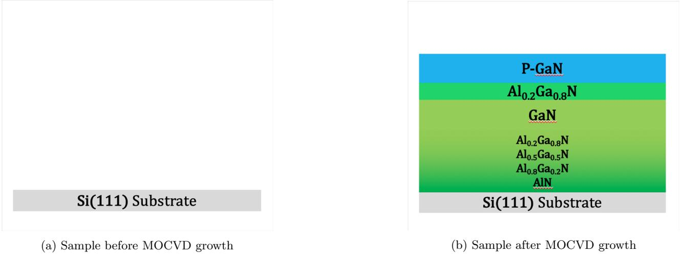
Figure 8: MOCVD growth of buffer layers, GaN layer, AlGaN layer and PGaN layer
