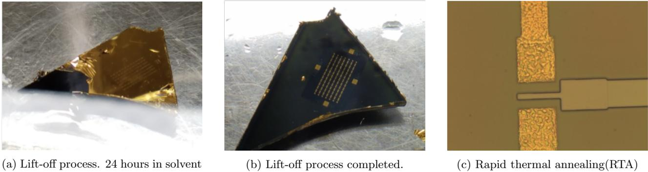
Figure 13: Lift-off and RTA of Ohmic contacts
