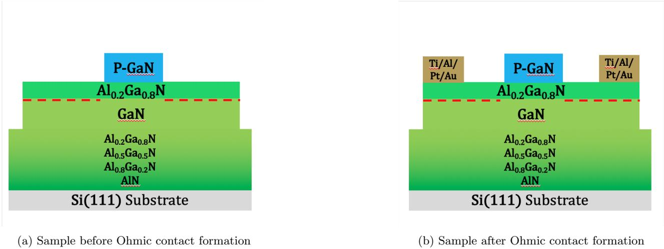
Figure 12: Ohmic contacts formed for the source and drain contacts
