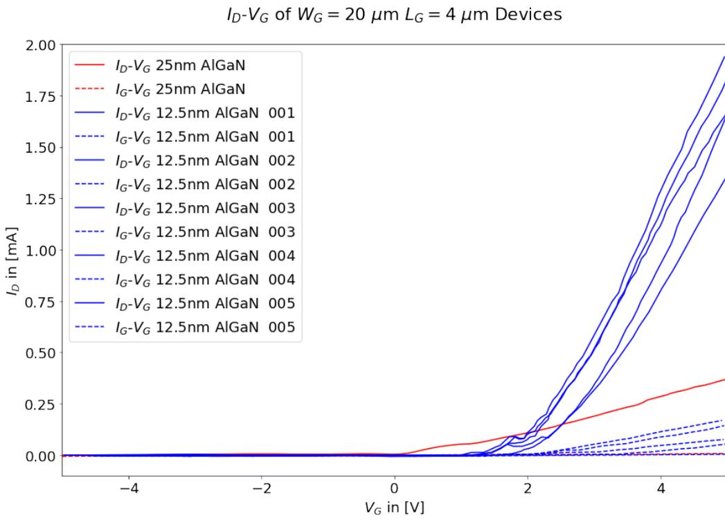
Figure 18:  $I_D - V_G$  and  $I_G - V_G$  curves of our  $20 \mu\text{m}$  width devices.  $V_{DS} = 5 \text{ V}$ . The original data csv files were lost, so those data were retrieved from the pictures of the plots taken during the measurement with graph-reading applications.
