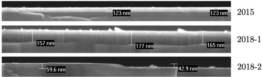
Figure 16: PGaN thickness measured at different times.
