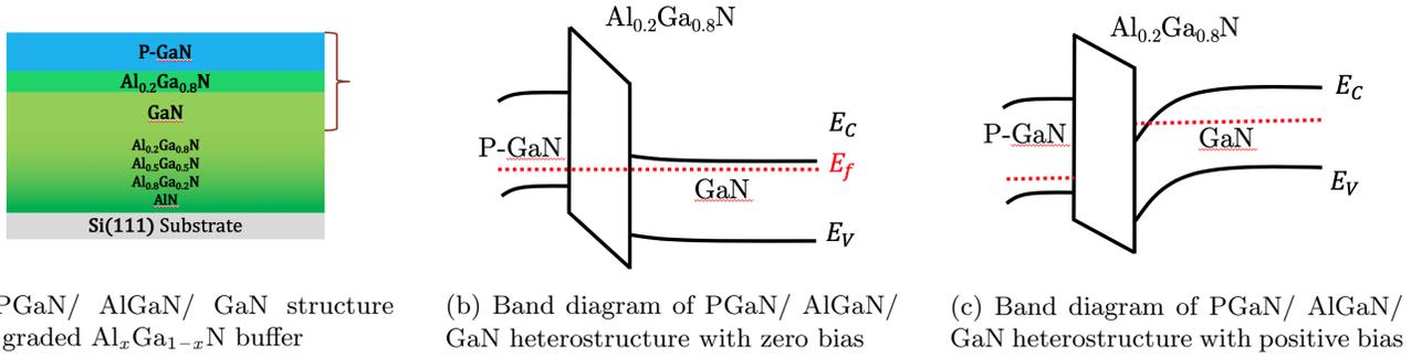
(a) PGaN/ AlGaIn/ GaN structure with graded  $Al_xGa_{1-x}N$  buffer
