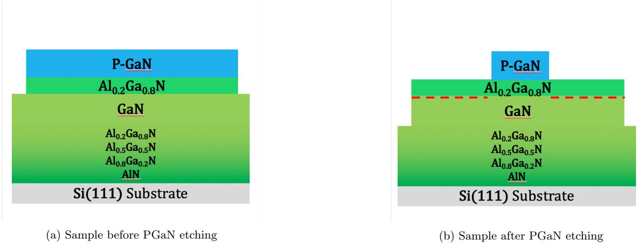
Figure 10: PGaN etching to leave PGaN layer only for the gate area
