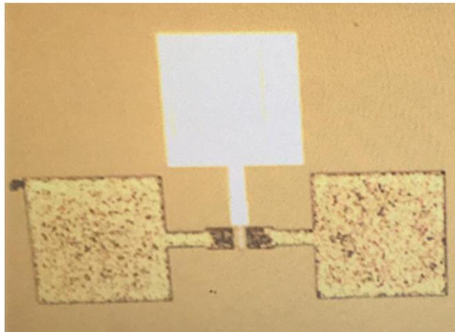
Figure 15: Schottky contact formed(white metal)
