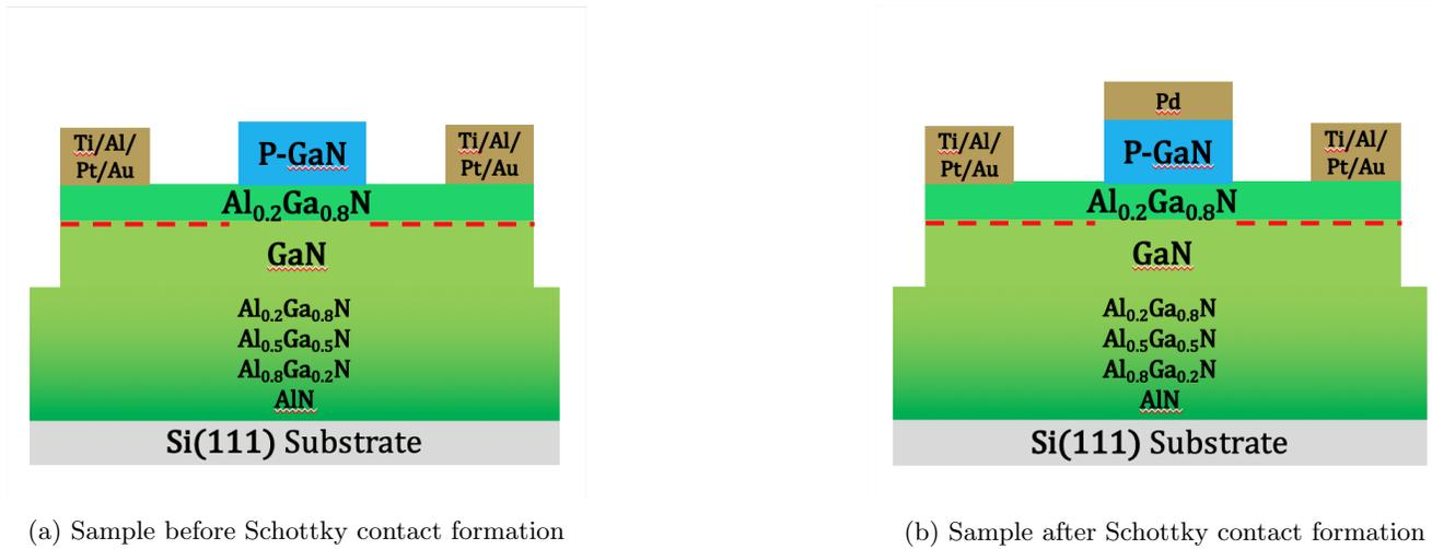
Figure 14: Schottky contact formed for the gate
