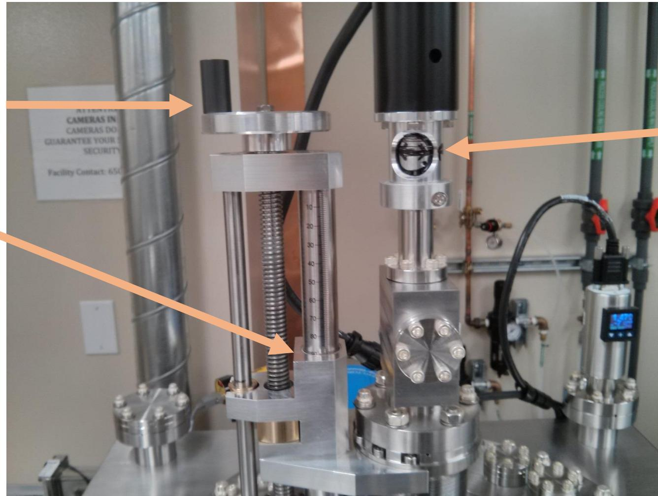
2) Rotate the inner cylinder with your hand until you see the double arrow in the window.
