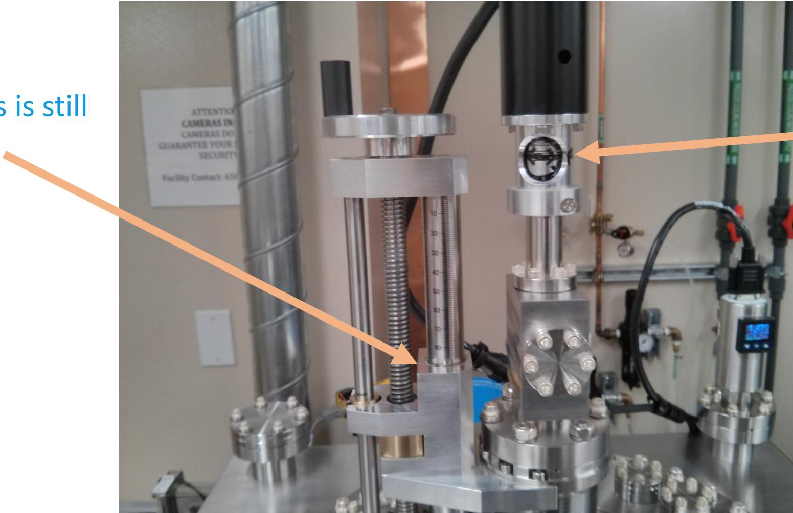
2) Rotate the inner cylinder with your hand until you see the double arrow in the window.
