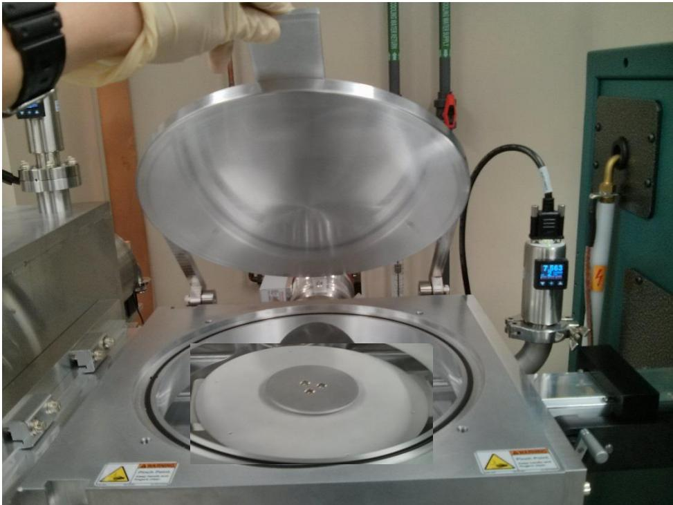
2) Hold chuck from the backside and remove from load lock.
