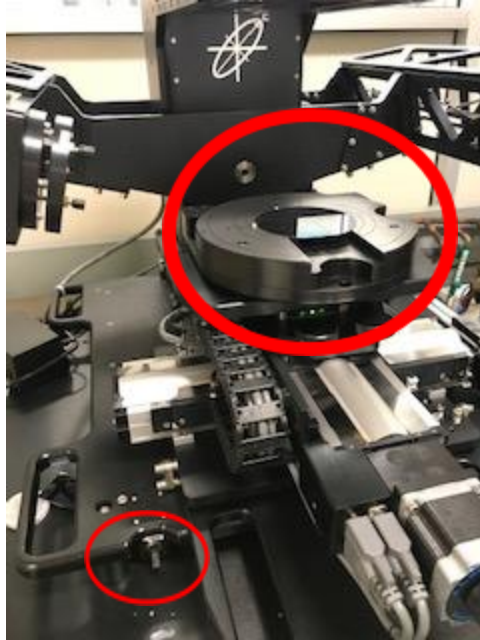
Figure 2: Location of vacuum switch, lower left corner. Sample stage upper right.
