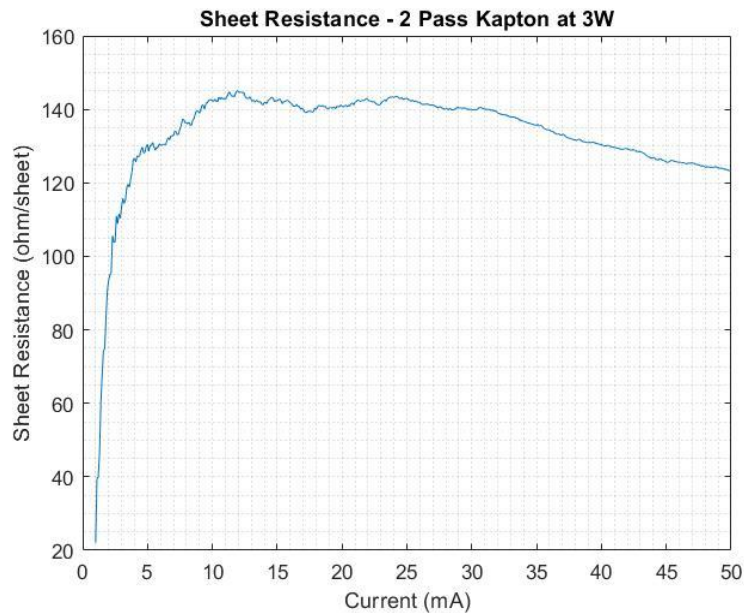
Figure 12: Sheet resistance curve for 2 Pass Kapton sintered at 3W, with copper wire setup
